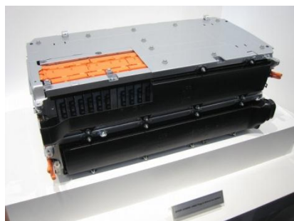
写真1 SPORT HYBRID i-MMD Plug-in lithium-ion battery (本田技研工業)
